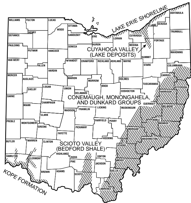
Areas of Ohio subject to severe slope failure.
