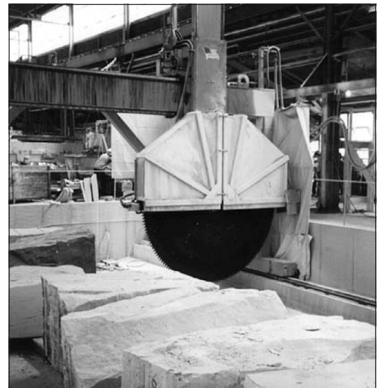
Diamond-tipped blade of a circular saw cuts sandstone into dimension stone
